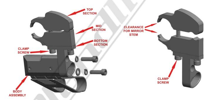
**STEP 1** - The BODY ASSEMBLY must be removed to gain access to the CLAMP SCREW. Remove the two socket head screws as shown above. Be sure to remove the lock washer with the top screw along with the lock washer and flat washer with the bottom screw.
