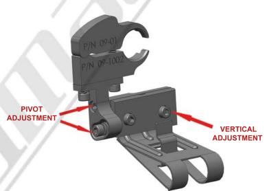
STEP 6 - Install your radar detector onto the mount. Use the adjustments shown above to adjust the RD to your desired position. We recommend adjusting the RD as close to the bottom of your mirror as you can. Be sure to tighten all adjustment screws after the adjustments are made.
