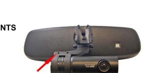
SPRING CLIP HORIZONTAL **ADJUSTMENT SCREW**
