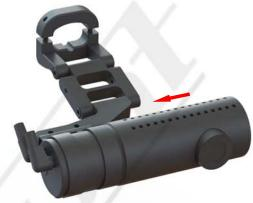
1 - To install the dashcam into the mount, simply squeeze the two tabs of the spring clip together as shown above. This will increase the diameter of the spring clip and allow you to slide the dashcam into position. Once the dashcam is in position, release the two tabs. The dashcam is now securely attached to the mount.
