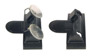
STEP 1 - Remove the two suction cups that are on your existing V1 windshield mount. The two holes that were used to secure the suction cups are now used to attach the BlendMount.
