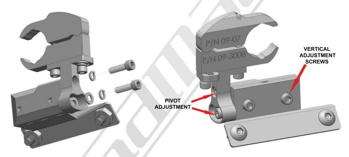
STEP 7 - Reinstall the BODY ASSEMBLY. Be sure to include the lock washer with the top socket head screw and the lock and flat washer with the bottom socket head screw as shown above. NOTE: there are extra lock and flat washers included in the tool kit just in case you happen to misplace one.
