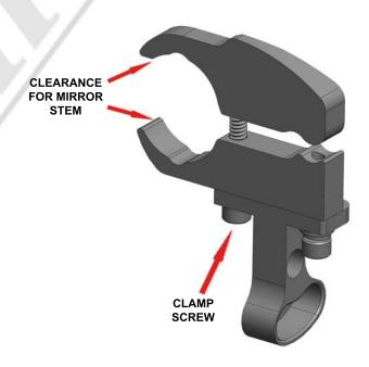
STEP 4 - Loosen the CLAMP SCREW so there is enough clearance between the TOP and MID SECTIONS to slide over the mirror stem.
