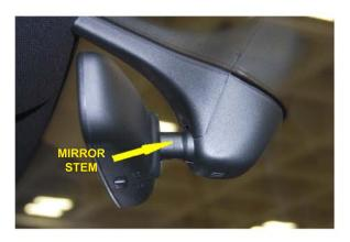
**STEP 5** - While sitting in the passenger seat, place the mount over the mirror stem. Tighten the CLAMP SCREW until the mount starts to clamp onto the mirror stem. Position the mount as far forward as it will go and paralell to the bottom of the mirror before fully tightening.
